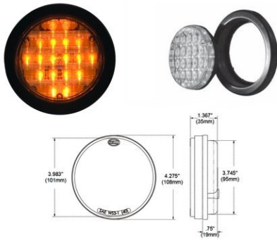
Model EXL 400 4" Warning Lamp 12/24V round amber LEDs clear lens
